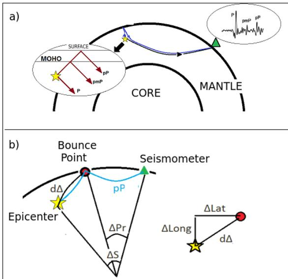
**Figure 2:** a) Reflection of the P wave from the underside of the Moho (pmP) and surface (pP), drawings modified from McGlashan et al. 2008. b) Bounce point localization.
